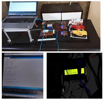
• HARDWARE TESTING: When making pcb there is shorted two paths accidentally because of which we are getting output the error while we tested for continuity. While making power supply we are not getting desire output so we check voltage at every point then we found error in the capacitor then we change it and then capacitor got desire output.
