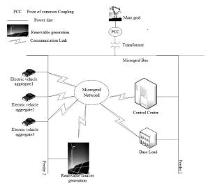
The microgrid and main grid are linked together via a common coupling (PCC). The microgrid consists of the base load, the renewable energy storage, the control center and other generators and EVs. Wind turbines and solar panels are generating renewable energy. Base load refers to a load that excludes the load of an electric vehicle.
